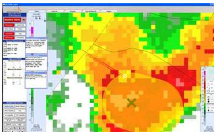
Fig. 4. Example of display showing a microburst affecting an airport using a dedicated aviation weather decision support system (Barrere et al., 2008).
