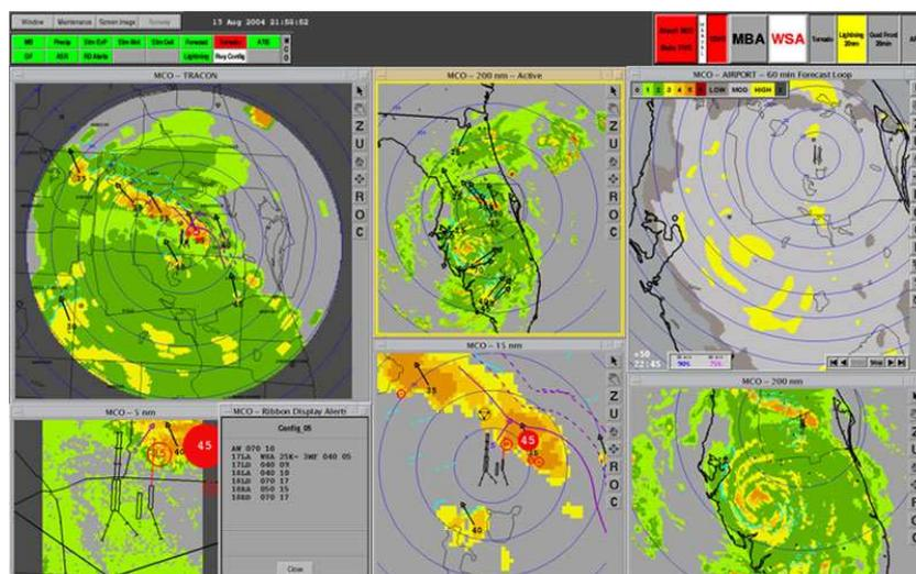
Fig. 5. Display of ITWS system that provides multiple views of weather round an airport (<http://www.ll.mit.edu/mission/aviation/>).
