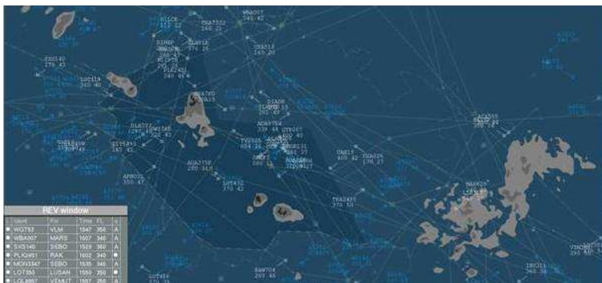
Fig. 1. Example of ACC display with radar MAX data (ATRAK system).
