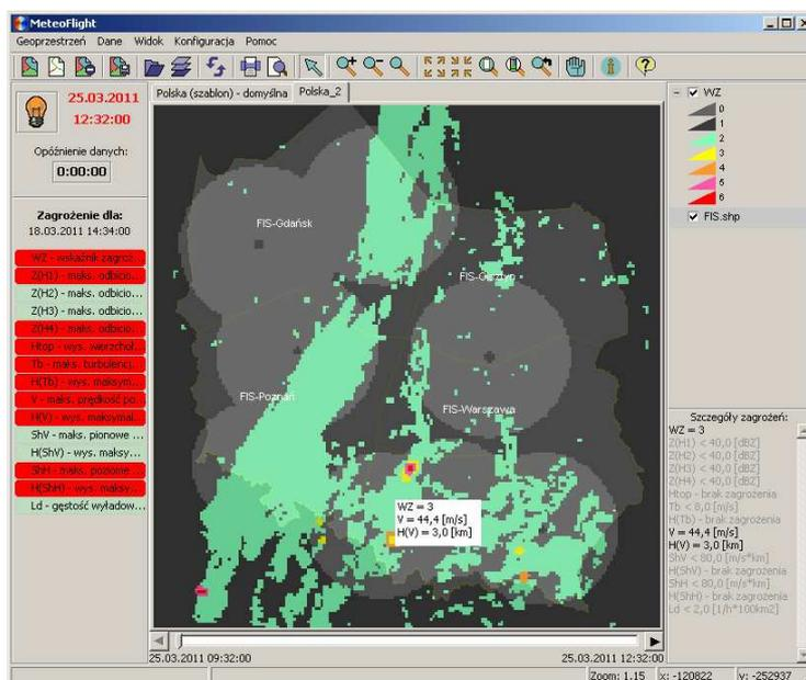
Fig. 6. Weather hazard index displayed by MeteoFlight application.
